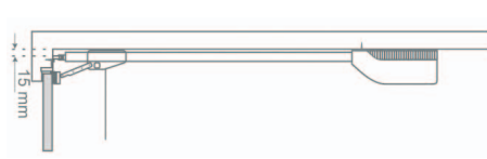
▲ Guide rail mounted to the ceiling and lintel.
